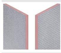
**SUPERCEL® AERIS** comprises a high performance rigid thermoset with a **phenolic resin insulation core** autohesively bonded with an **aluminum vapor barrier foil facer** on the upper side and a **micro-perforated aluminum foil facer** on the lower side.
