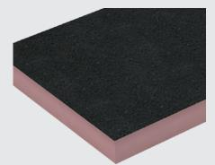
**SUPERCEL® FLAMMA** is a high performance rigid thermoset with a phenolic resin insulation core, a mineral added paper based facing covering one side and a graphite based membrane covering the other side. The latter facing should be placed on the side that risks being exposed to flames, guaranteeing both high fire performance and hydro-repellency.
